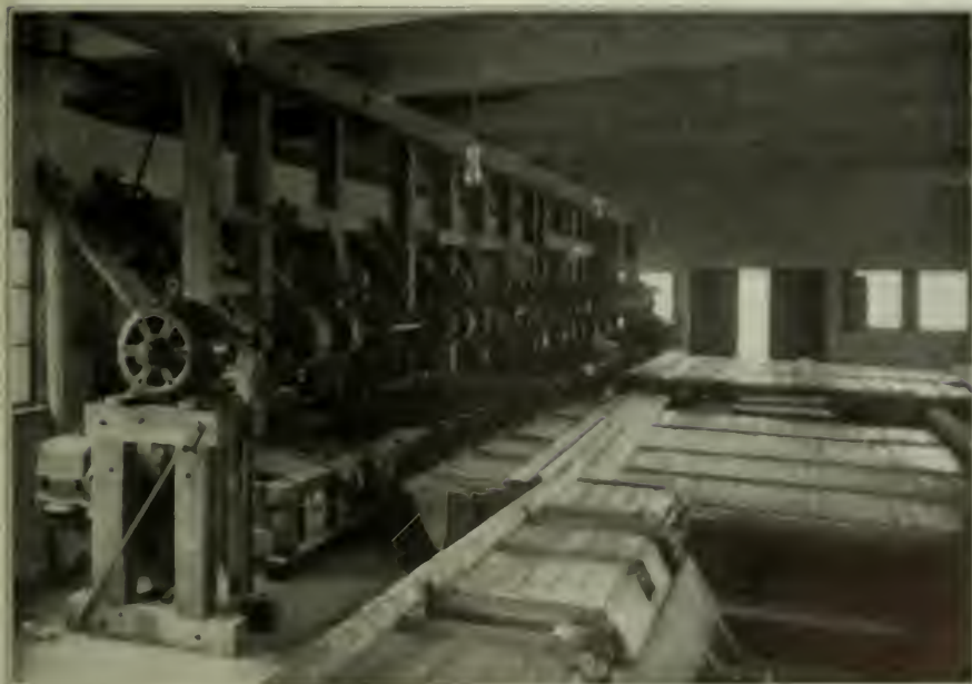
FIG. 2. TRIMMERS DRIVEN BY 20-HORSEPOWER MOTOR
